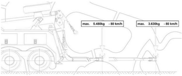
Suspendable towing weight increases, when speed is reduced.
