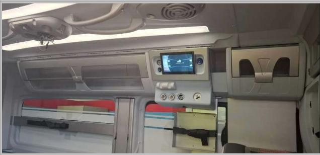
Front wall cabinet, position A, made of FCS (Fiber Composite Spraying) polyurethane, shockproof, 450mm long with pressure opening, internal lighting, door equipped with glass for easy identification of the material.
