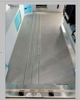
Fitting at the rear and side profiles of the flatbed of non-slip, rice grain aluminum door sills, designed to prevent wear and tear of the floor at the up/down points, most subject to wear and tear
