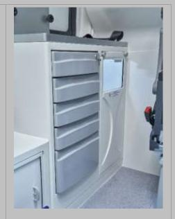
Wheel arch cover structure, with compartment closed by sliding door
