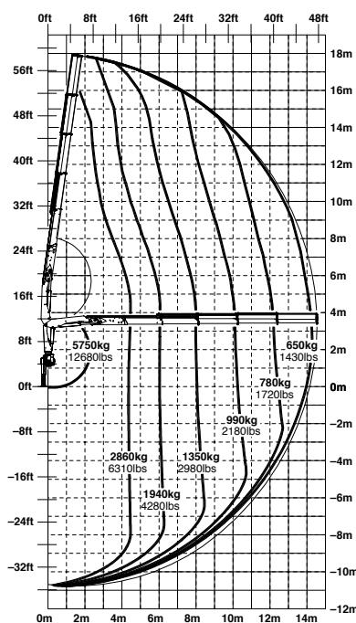
The reaches are indicated for a 20° main boom position and are therefore not the maximum ones.
