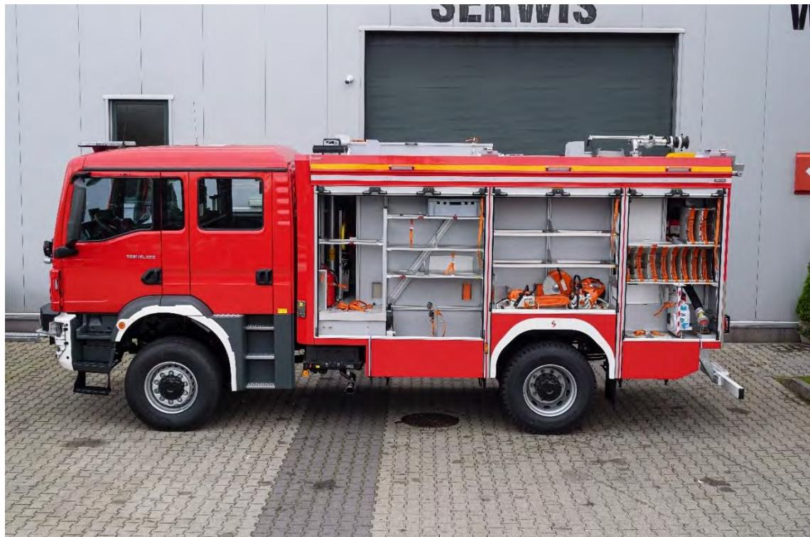
In the front part of the structure there is space for long elements that are often used during operations. There is a mount for medical equipment such as a stretcher, Kramer splints or a medical bag. The front compartment has a retractable panel with a mount for two Breathing Apparatus cameras and a drawer with a power generator.
