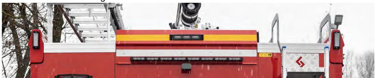
5. The vehicle is equipped with additional reverse gear lighting on the rear wall and under the cabin steps.
