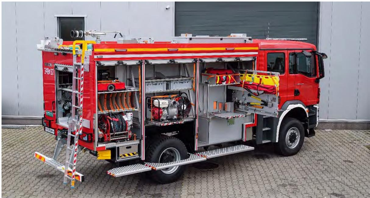
Under each compartment there are tilting platforms, including two tiltable ones in the form of vehicle wheel arches. **The design of the steps ensures their load capacity of 280 kg**. Each step has additional LED warning lighting on the edge or a gelcoat finish.
