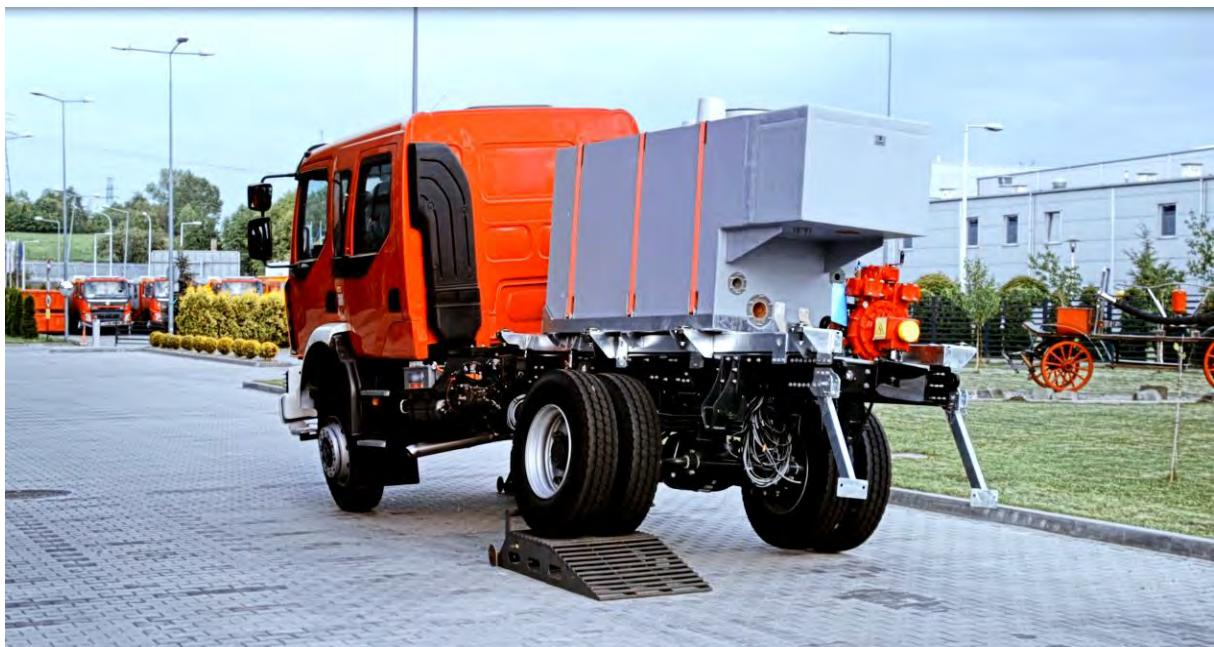
The structure is made in a 3+3+1 compartment system, which ensures maximum equipment capacity, ensuring a depth of 600 mm in each compartment.
