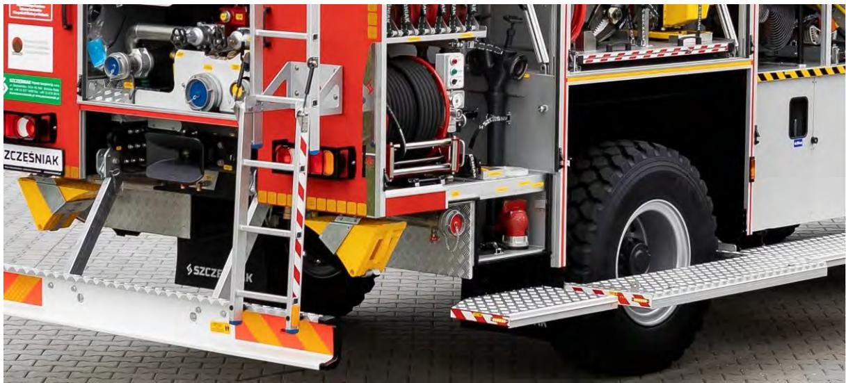
**Sprinkler system** installed in the chassis to limit chemical contamination zones or for fire-fighting purposes, equipped with 4 nozzles with a capacity of 50 dm<sup>3</sup>/min. each. Two sprinklers placed in front of the front axle, two sprinklers on the sides of the vehicle. Sprinklers are made of brass.
